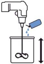
Mix rubber material in can/pail until uniform; center mixer shaft in pail or can and begin mixing until a vortex is formed. Slowly pour all of catalyst into vortex. Move mixer up and down and in a circular motion for 2-3 minutes until all portions of can/pail are uniformly mixed.
